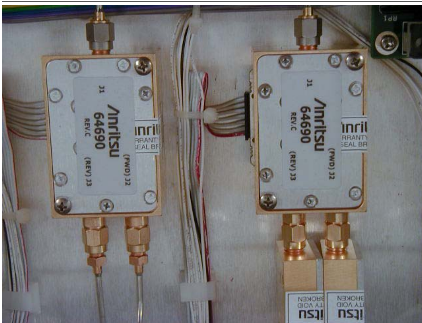
Figure 5-9. Low Band Switches (A5 is shown on the left and A6 is shown on the right)
